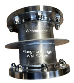
WA-wall-sleeves Flange to Flange models cast in new concrete walls for pipe passage through the foundation. Inbound pipes bolt directly to the flange. Nuts on the back of the flanges are protected from concrete residue.
